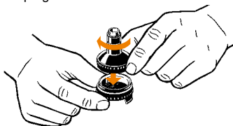
Screw on Filling Chamber Cap
